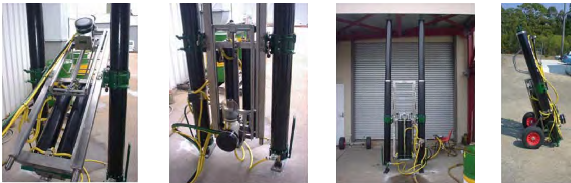
Pictured: High Seam Drill 2000, the two Stinger Legs allowing the drill to be rotated through 360°
